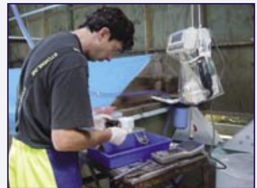
Calibrating sea urchin roe color with a Minolta Spectrophotometer interfaced with Allegro CE/DOS.
